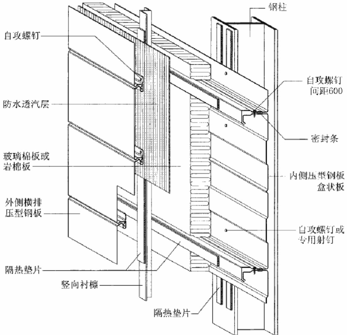
**双层压型钢板复合保温墙体（外板横排）构造**
