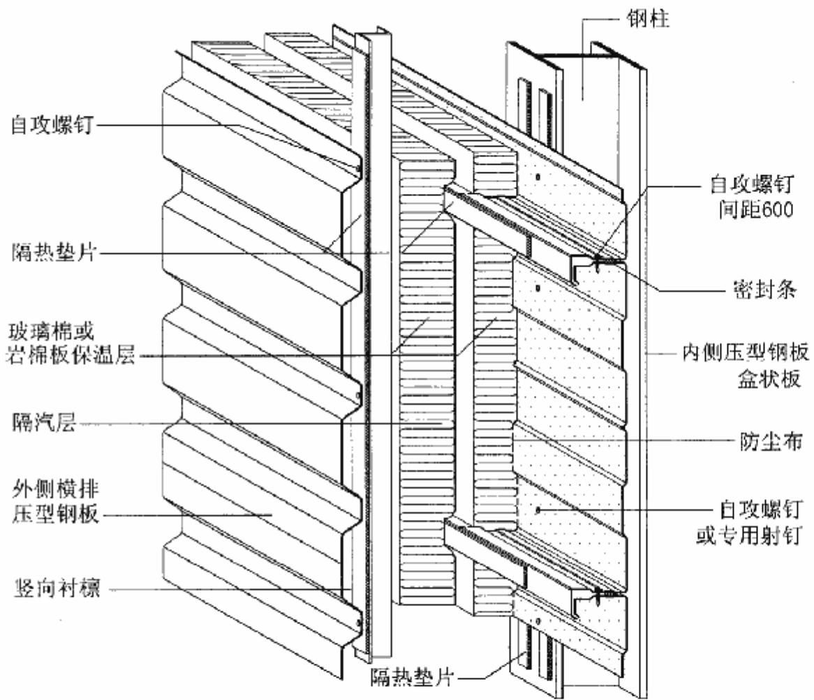
墙T2-压型钢板复合保温吸声墙体（外板横排）构造
