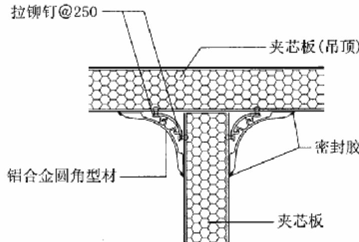
1 隔墙与吊顶连接
